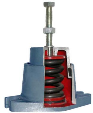
Spring PHONOLATOR type A5/85 housing of light metal cast iron, with height-adjustment device and body noise-damping coat, can be loaded from 100 to 165 kg, for speed above 630 rpm
