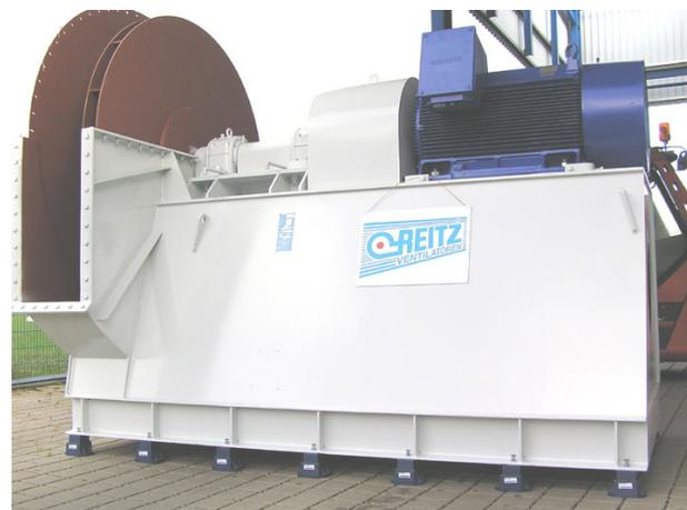
III.10: Vibration-isolated set-up of a fan,
